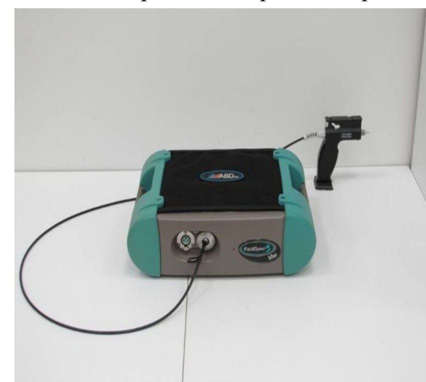
Figure 2. ASD FieldSpec 3 MAX portable spectroradiometer
